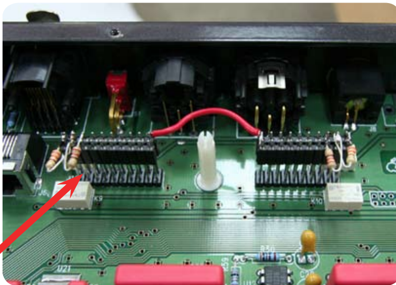
Header with resistors installed plugs into pins
